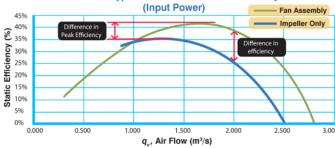
It should also be noted that the tests performed by the motorised impeller manufacturers are completed using their purposely-designed inlet cones and are set to have an ideal overlap between impeller and inlet cone. To reduce production costs many of the local fan manufacturers use their own inlet cones which suit a variety of their fan ranges. These inlet cones often do not follow the supplier's overlap recommendations, thereby further reducing performance.
