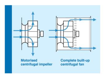
Fantech recently undertook testing to determine the actual differences in performance between a motorised centrifugal impeller-only assembly and a built up centrifugal fan in a housing. At a given duty point the results are as follows:
